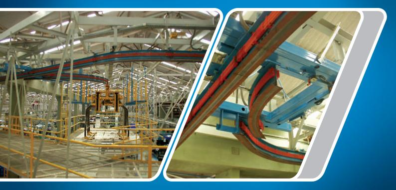
An intelligent conveyor system, a solution to all complex requirements of material handling which includes transfer of components at variable speeds on the same line, integration with other transfer system and devices with utmost accuracy and precision and controlled vertical movements of carriers.
