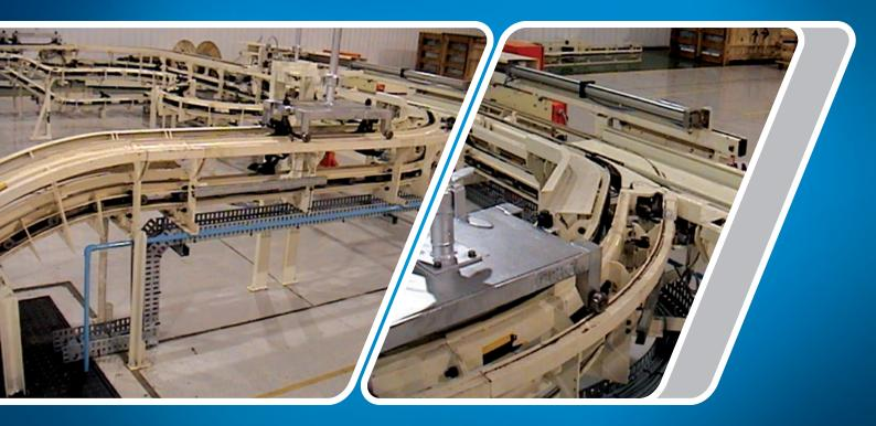
The inverted power and free system is designed to offer to the customers all the features of an overhead power and free conveyor along with the robustness and operational consistency of a regular skid conveyor system.
