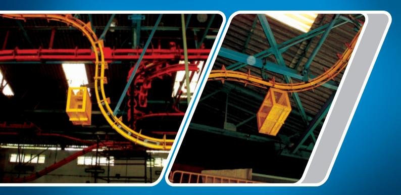
A specially designed; modular and flexible power only (trolley) conveyor system which uses the bi-planar chain to offer versatility and suitability for use in steel and plastic parts painting lines apart from the general applications.
